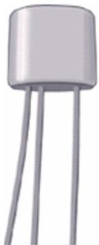
A transistor mounted on a metal can with three wires to each of the three terminals.
